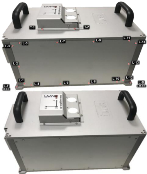
Figure 5. The iCORUS reference points (markers) given in Table 1 and coordinate axis directions on the top of the IMU.
