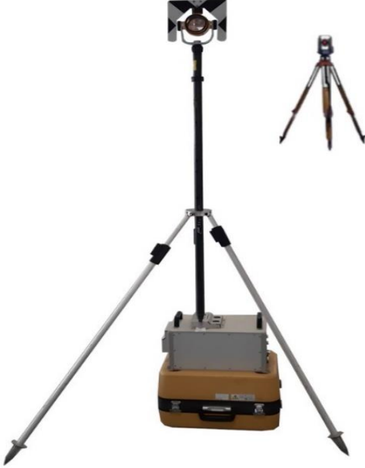
Figure 4. Experimental setup with IMU, reflector, and total station.
