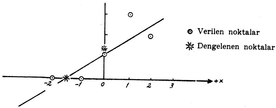
$$\begin{array}{lcl} a x_1 + b - y_1 = v_1 & & -2a + b - 0 = v_1 \\ a x_2 + b - y_2 = v_2 & & -1a + b - 0 = v_2 \\ a x_3 + b - y_3 = v_3 & & 0 + b - 1 = v_3 \\ a x_4 + b - y_4 = v_4 & & 1a + b - 3 = v_4 \\ a x_5 + b - y_5 = v_5 & & 2a + b - 2 = v_5 \end{array}$$
