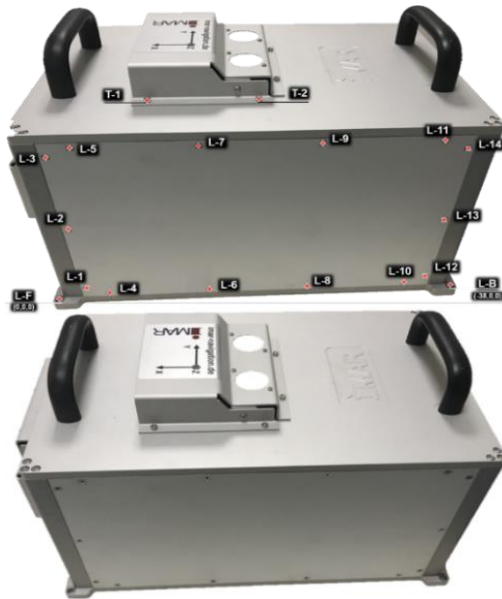
Figure 5. The iCORUS reference points (markers) given in Table 1 and coordinate axis directions on the top of the IMU.
